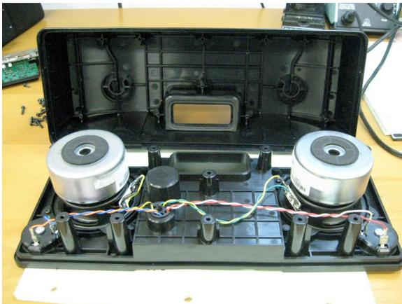
Figure 5: Acoustic housing disassembled. The woofers share a rear acoustic chamber. Production units have foam around the wires to prevent buzzing.
