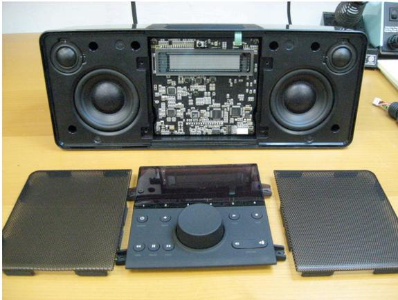
Figure 3: Grills and front panel removed.
