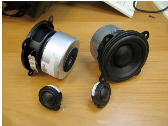
Figure 6: Loudspeaker Drivers. Each channel uses a woofer and tweeter
