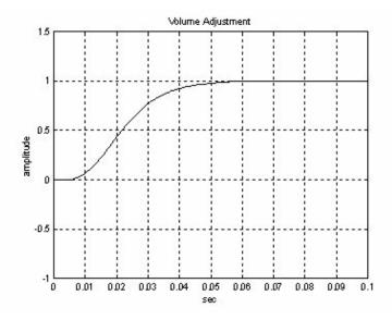
Figure 9: Click-less volume changes in Squeezebox Boom. This volume ramping profile shows how the volume gently changes from one volume to another. This shows a switch from 0 to 100% volume, but any other volume change follows a similar.
