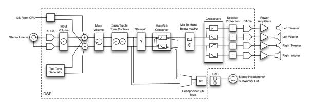
Figure 8: Block diagram of the Squeezebox Boom DSP flow (with other components for reference)
