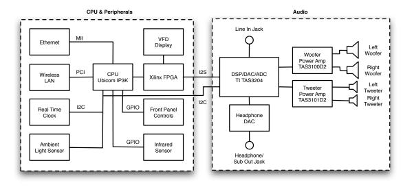
Figure 1: Squeezebox Boom Block Diagram. This paper will discuss the audio design, starting at the I2S & I2C interface between the CPU and Audio sections and follow the signal path through to the speakers, line-in and subwoofer-out.
