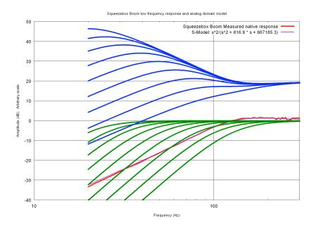
Figure 12: Family of low-frequency equalization curves (blue) and simulated low-frequency system response (green). The curves show cutoff frequencies ranging from 20Hz to 137Hz in 1/3-octave steps. For clarity, the blue curves are offset by +20 dB. The green curves correspond to the final overall frequency response of the system (simulated in this figure). They are  $4^{th}$ -order Linkwitz-Riley high pass filters.
