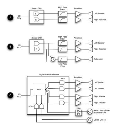
Figure 7: Comparison of different desktop speaker architectures.
