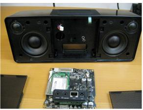
Figure 4: Main board removed, exposing the rear of the main board and acoustical chamber.
