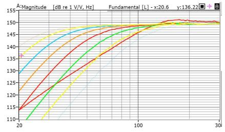
Figure 11: Actual in-box frequency response measurements of the family bass extension filters used in Squeezebox Boom.
