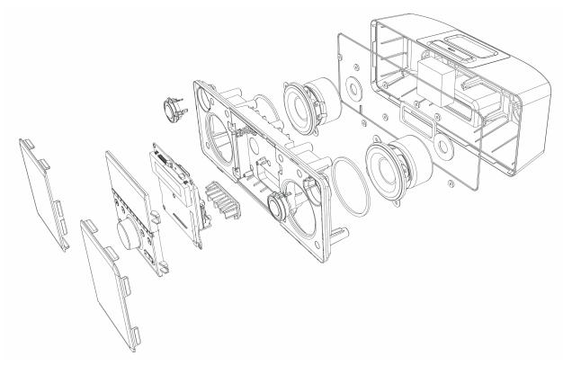
Figure 2: Exploded schematic view of Squeezebox Boom assembly
