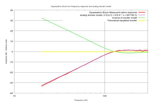
Figure 11: Frequency response of Squeezebox Boom, with theoretical low frequency compensation filter. Red: Measured response; Blue: theoretical model; Green: compensating filter; yellow: Theoretical frequency response of the equalized system.
