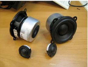
Figure 6: Loudspeaker Drivers. Each channel uses a woofer and tweeter
