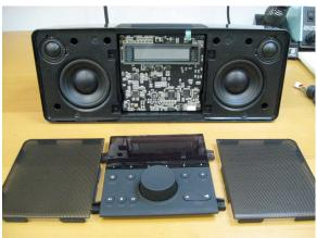
Figure 3: Grills and front panel removed.
